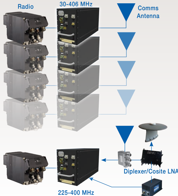
Typical Command & Control Platform (Multi radio systems)
