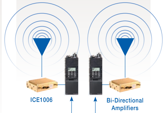
Comms Radio Relay (Retrans)
